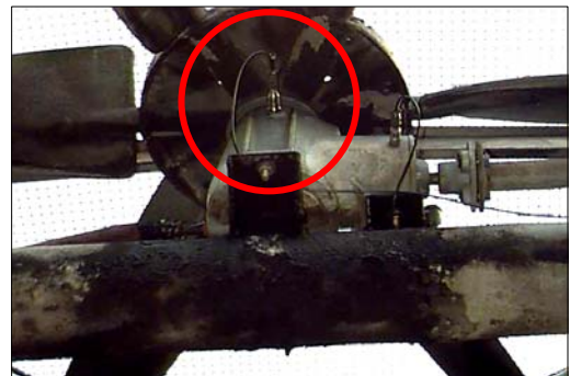
View of a large-cell fan from below, showing the mounting of a 799LF low-frequency accelerometer on the side of the gearbox.
