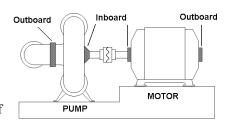
horizontal position at each bearing (4) and one in the axial direction at the inboard pump bearing (1) for the total of five (5).
