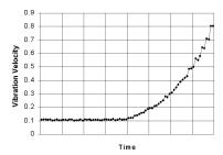
Trending the rate of increase in vibration can also be a useful measure of machine condition.
