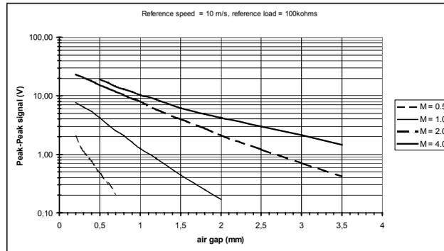
Typical signal amplitude with ferromagnetic gear.
